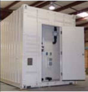
SC20 shipping container treatment units
